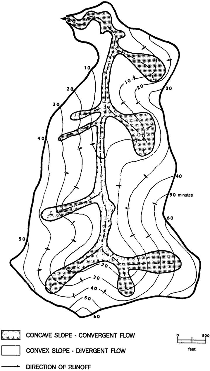
Figure 5. Flow Zones and Runoff Travel Times.
