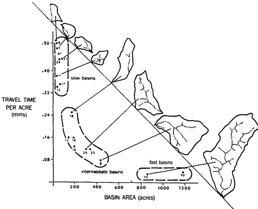
Figure 4. Travel Time Per Acre of Drainage Area. Small basins where a large part of the runoff is made up of overland flow are much slower per acre than large basins where channel flow is the primary mode of conveyance.
