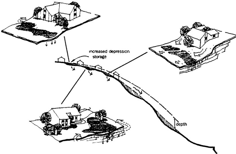
Figure 8. Vegetative Buffers Integrated with Depression Storage in Residential Areas on Upland Surfaces. Most lots of 0.25 acres or larger can easily detain the first 0.5 inches of runoff on site.
