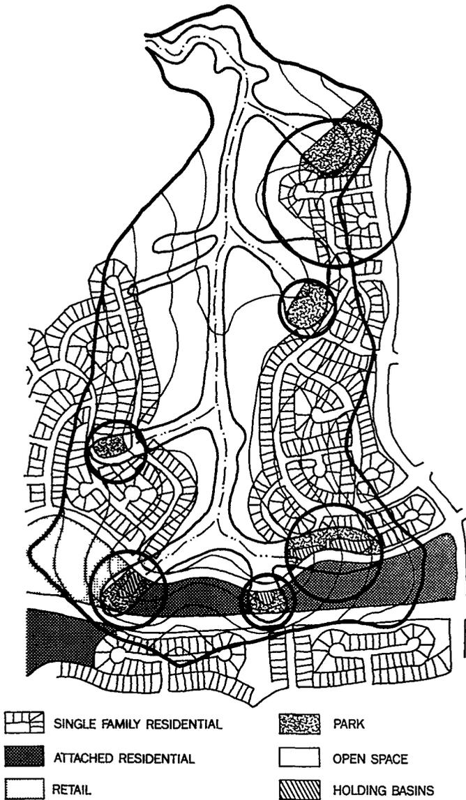
Figure 7. Modified Land Use Plan Integrating Park/Open Space and Stormwater Management. Each zone of convergent flow is used for water management. The overall balance between park and single-family residential acreage remains the same. The area taken from attached residential and retail would total about three acres.
