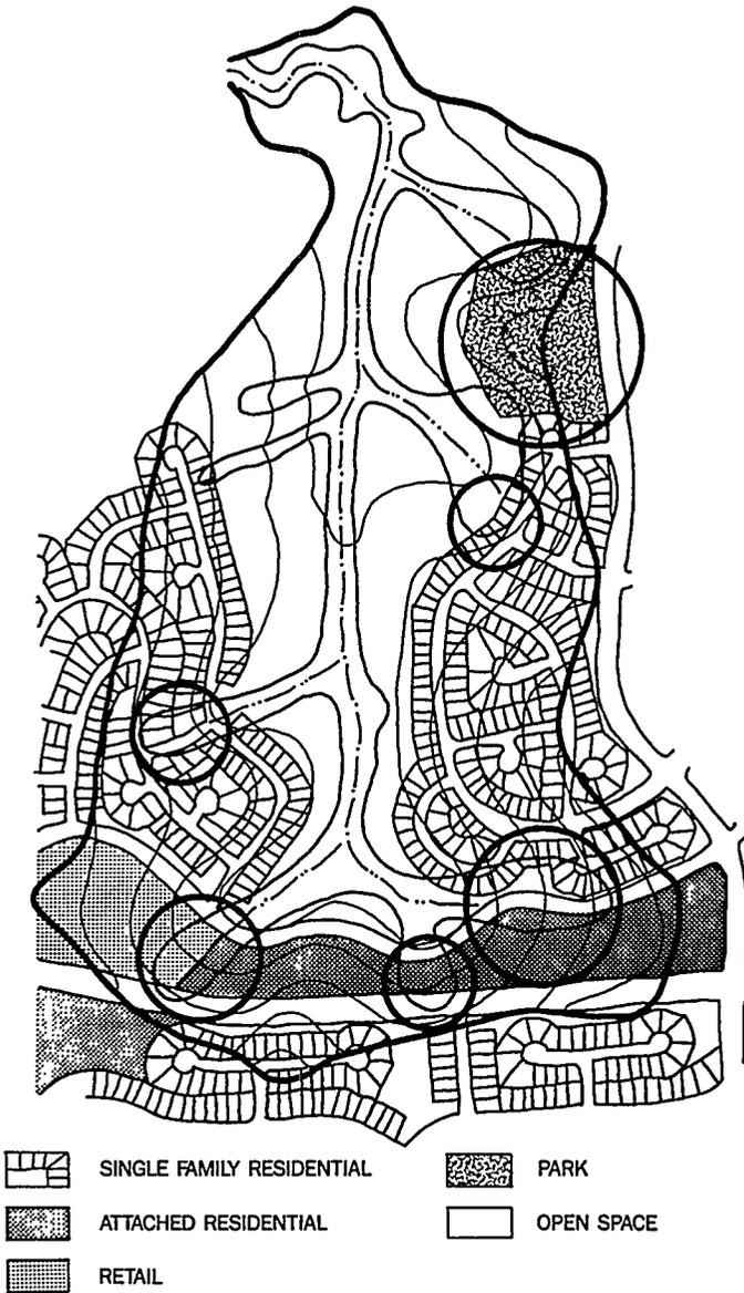
Figure 6. Inappropriate Land Uses Relative to Flow Zones (circled areas). An example in the upper right shows high density land uses in areas of convergent flow and open space (park) in an area of divergent flow.
