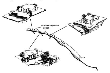
Figure 8. Vegetative Buffers Integrated with Depression Storage in Residential Areas on Upland Surfaces. Most lots of 0.25 acres or larger can easily detain the first 0.5 inches of runoff on site.
