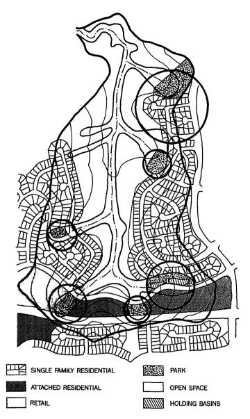
Figure 7. Modified Land Use Plan Integrating Park/Open Space and Stormwater Management. Each zone of convergent flow is used for water management. The overall balance between park and single-family residential acreage remains the same. The area taken from attached residential and retail would total about three acres.
