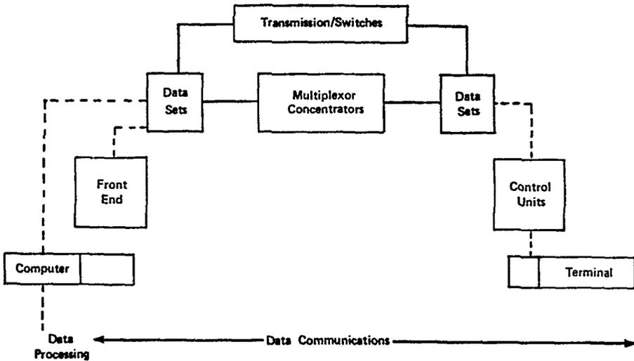
or any of a number of other media conversion devices. The terminal will be controlled by a control unit connected to a data set (or modem). The data set will be linked to a transmission channel which will then be connected to the computer shown at the extreme left.
